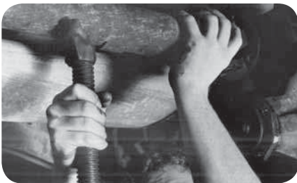
Support driveshaft (fig. 40).
