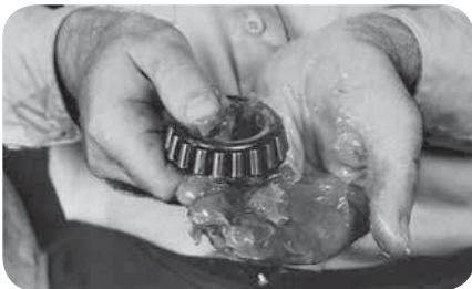
Grease bearing (fig. 7).
