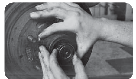
Install outer bearing (fig. 12).
