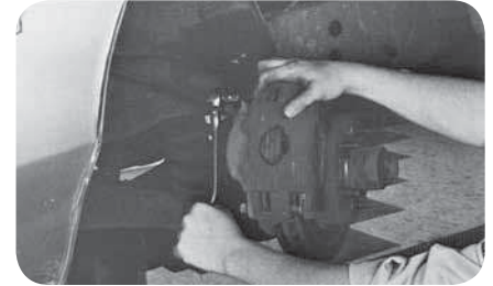
Loosen brake caliper mounting bolts (fig. 1).
