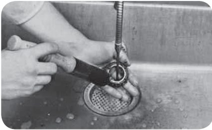
Rinse bearing in clean solvent (fig. 5).
