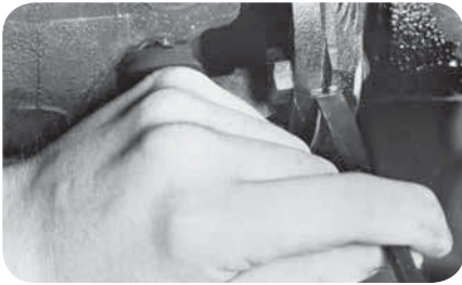
Mark the driveshaft and pinion flange (fig. 39).
