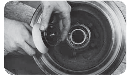
Slide SKF seal onto installation tool (fig. 9).
