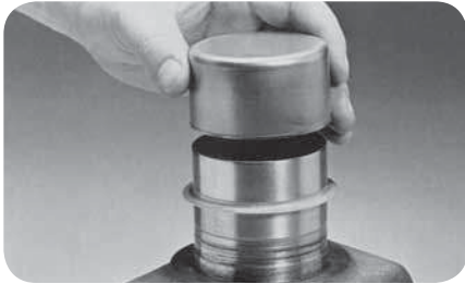
Place Installation tool over Speedi-Sleeve (fig. 46).
