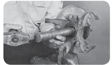
Chrysler – Remove hub from knuckle (fig. 29).
