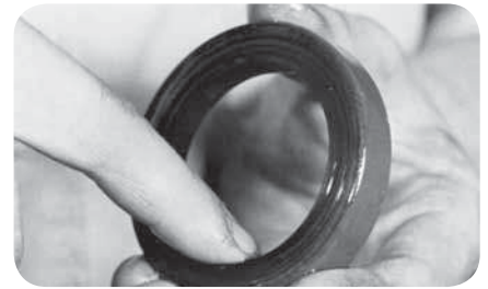
Apply lube to seal lips (fig. 43).
