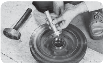
Place inner side of drum or rotor face up (fig. 8).
