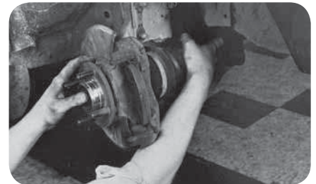
General Motors – Push shaft into hub (fig. 37).
