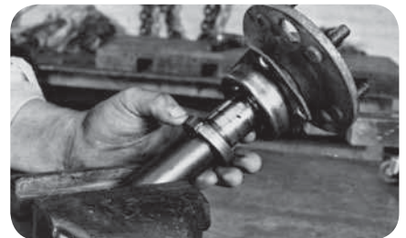
Slide off retainer (fig. 18).
